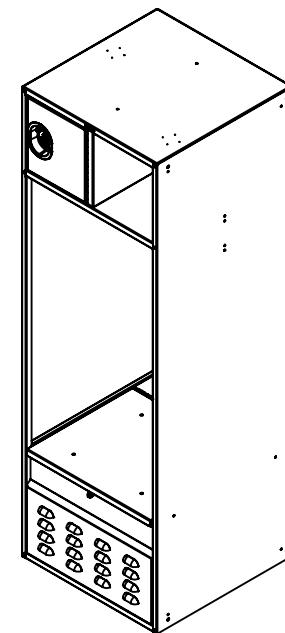
WELDED STEEL LOCKER, 24"W x 24"D x 72"H
