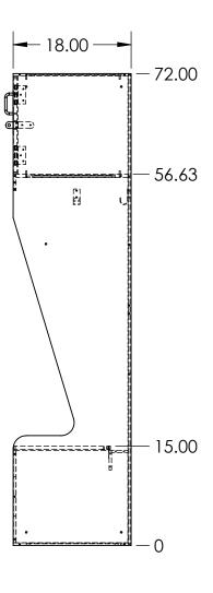
18X18X72 ATHLETIC CUTBACK VERTICAL VENT LOCKER MADE FROM VARYING THICKNESSES OF FORMICA COMPACT (PHENOLIC) MATERIAL
