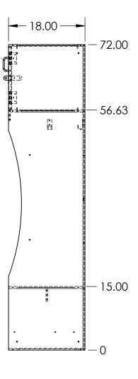
24X18X72 ATHLETIC RECESSED OPEN BOTTOM LOCKER MADE FROM VARYING THICKNESSES OF FORMICA COMPACT (PHENOLIC) MATERIAL
