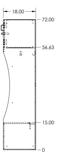
18X18X72 ATHLETIC RECESSED VERTICAL VENT LOCKER MADE FROM VARYING THICKNESSES OF FORMICA COMPACT (PHENOLIC) MATERIAL
