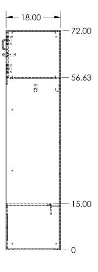
18X18X72 ATHLETIC STRAIGHT MESH GRILL LOCKER MADE FROM VARYING THICKNESSES OF FORMICA COMPACT (PHENOLIC) MATERIAL
