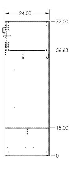
30X24X72 ATHLETIC STRAIGHT OPEN BOTTOM LOCKER MADE FROM VARYING THICKNESSES OF FORMICA COMPACT (PHENOLIC) MATERIAL
