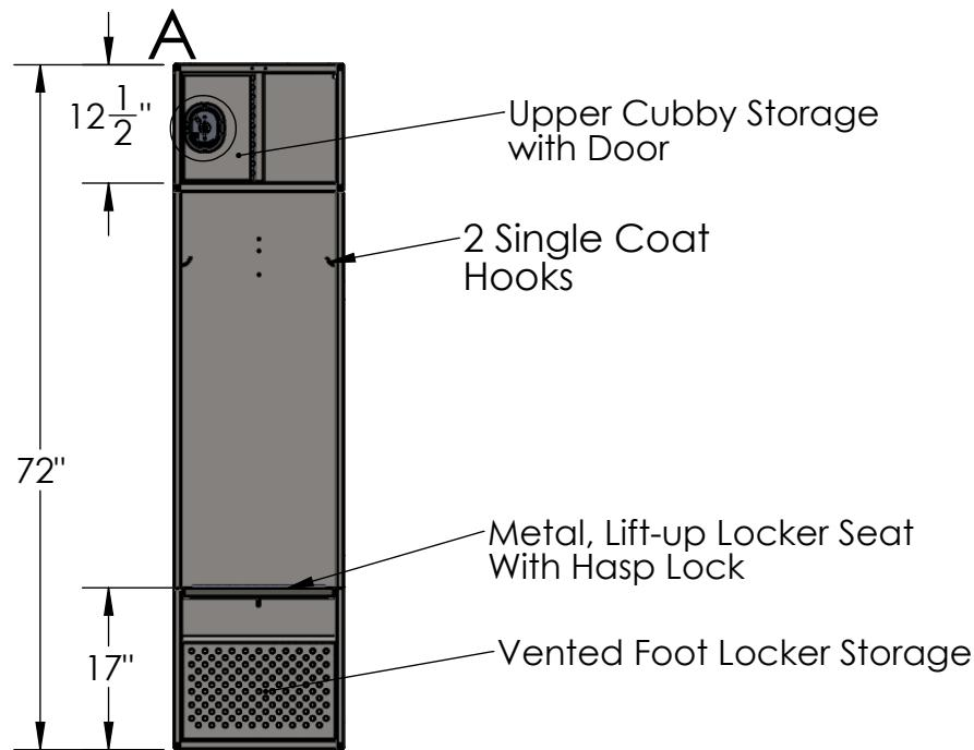
WELDED STEEL LOCKER, 24"W x 24"D x 72"H STANDARD FEATURES
