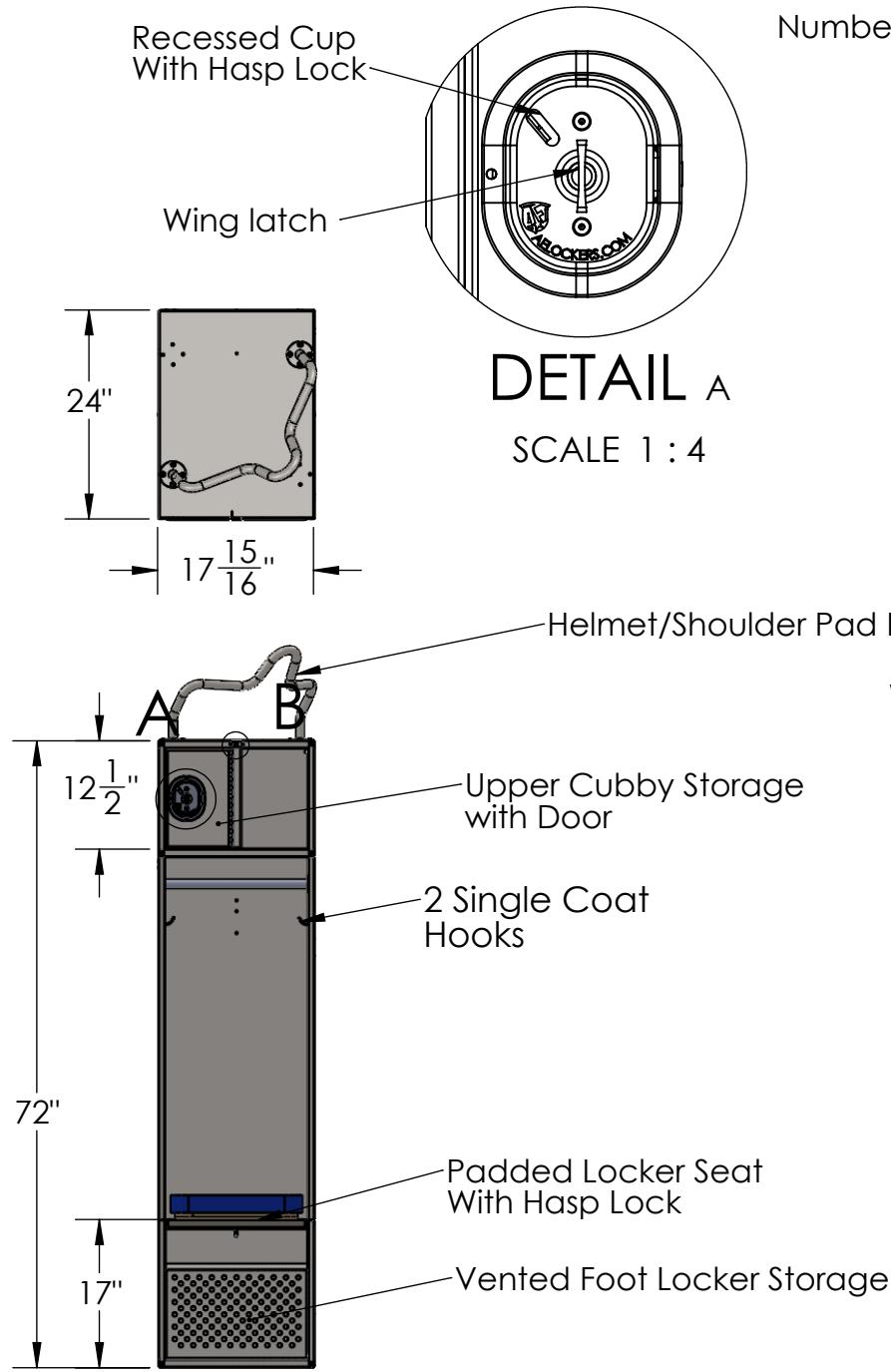
WELDED STEEL LOCKER, 24"W x 24"D x 72"H STANDARD FEATURES
