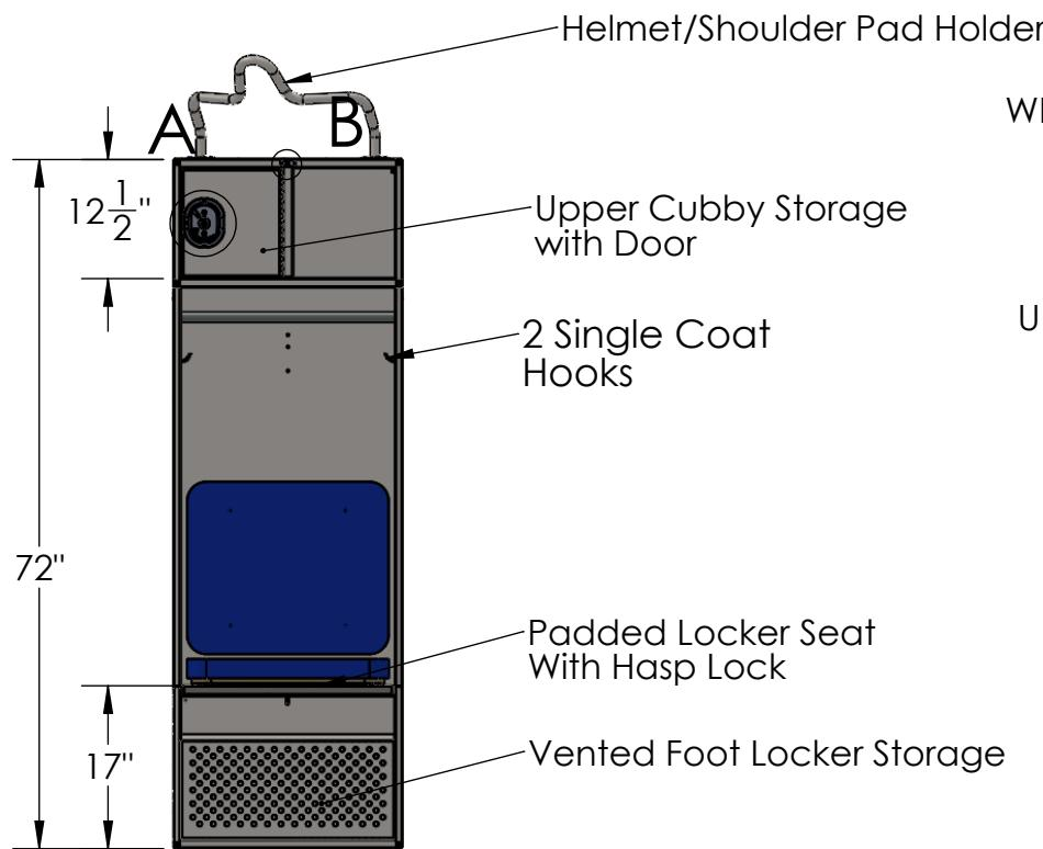
WELDED STEEL LOCKER, 24"W x 24"D x 72"H STANDARD FEATURES
